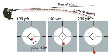
fig. 2a If the scope is mounted parallel to the bore, the path of a bullet will fall away from the line of sight due to the effect of gravity. The point of impact will, therefore, always be below the line of sight.
