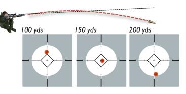
fig. 2b In order to account for this, the purpose of zeroing is to adjust the telescope so the barrel of the rifle is elevated in relation to it. The bullet path will then rise and fall through the line of sight, crossing first at around 25 yards. The point at which the bullet falls back through the line of sight is the zero distance, in this case 150 yards.
